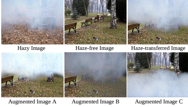
Figure 3. Illustration of PHDT-based hazy image augmentation. Beyond generating the haze-transferred image, we can apply gamma correction to F^{\text{TM}} to adjust haze density, either increasing or decreasing it to further augment images A and B. Additionally, we can vertically flip F^{\text{TM}} to augment image C.
