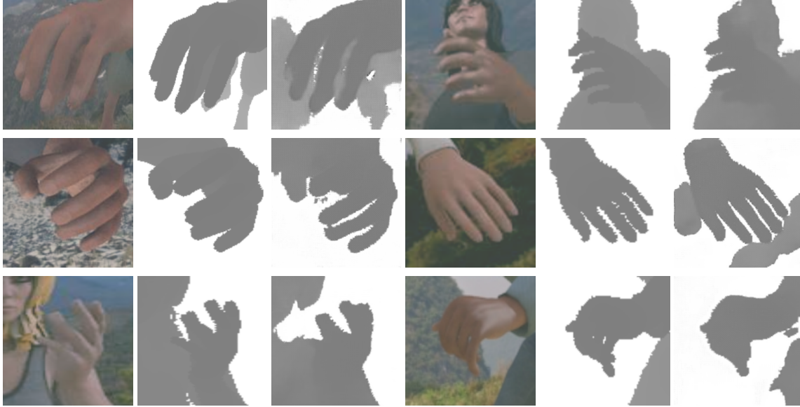
Figure 7. Comparison between the generated and ground-truth depth maps on the RHD dataset. The first and fourth columns show the RGB images. The second and fifth columns display the real depth maps. The third and sixth columns give the generated depth maps.
