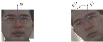
Fig. 7. Each image is divided into 96 regions. The distance between the two images is obtained when circularly shifting causes \psi' to be the new starting radial axis.
