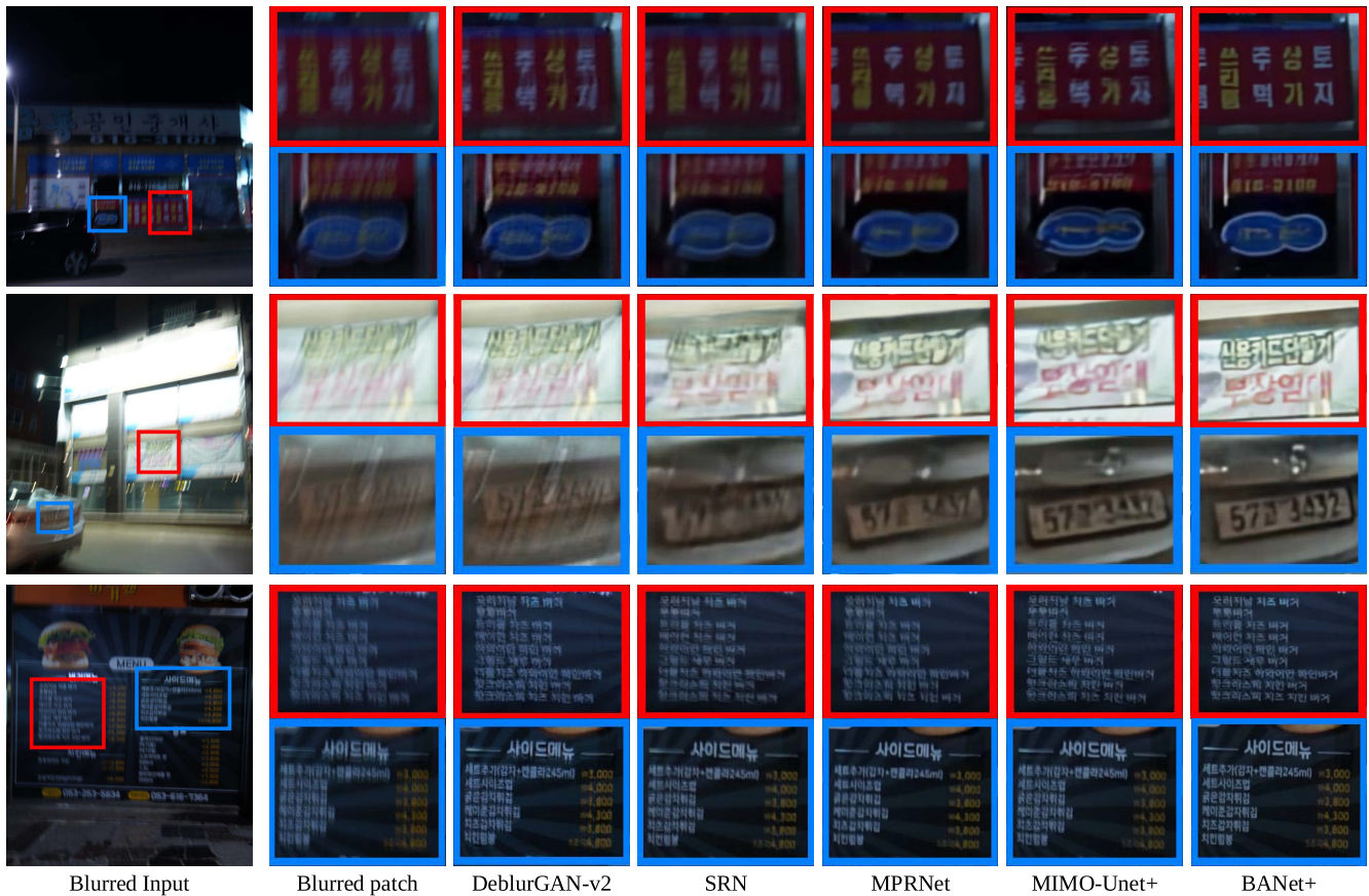
Fig. 13. Examples of deblurred results obtained using DeblurGAN-v2 [31], SRN [10], MPRNet [12], MIMO-UNet+ [34], and Ours on RealBlur [44] test set.
