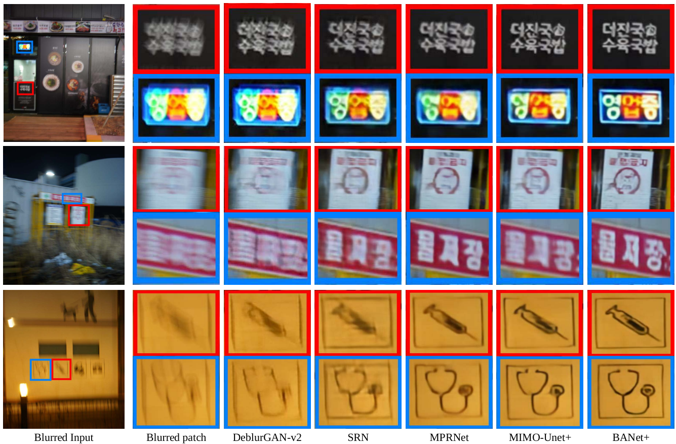
Fig. 12. Examples of deblurred results obtained using DeblurGAN-v2 [31], SRN [10], MPRNet [12], MIMO-UNet+ [34], and Ours on RealBlur [44] test set.
