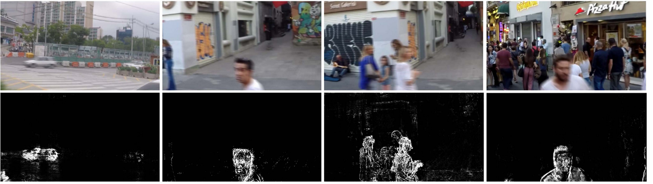
Fig. 8. Visualization of the blur-aware attended features on GoPro test set, where moving objects in the blurred images are highlighted while background is mostly excluded. These blur-aware masks are crucial for handling blurred images with diverse blur patterns.
