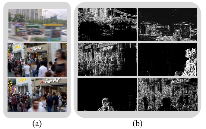
Fig. 7. Three disentanglement examples of blurred patterns of different degrees using our BA on GoPro test set. (a) Input blurred images and (b) attended feature maps on different regions.
