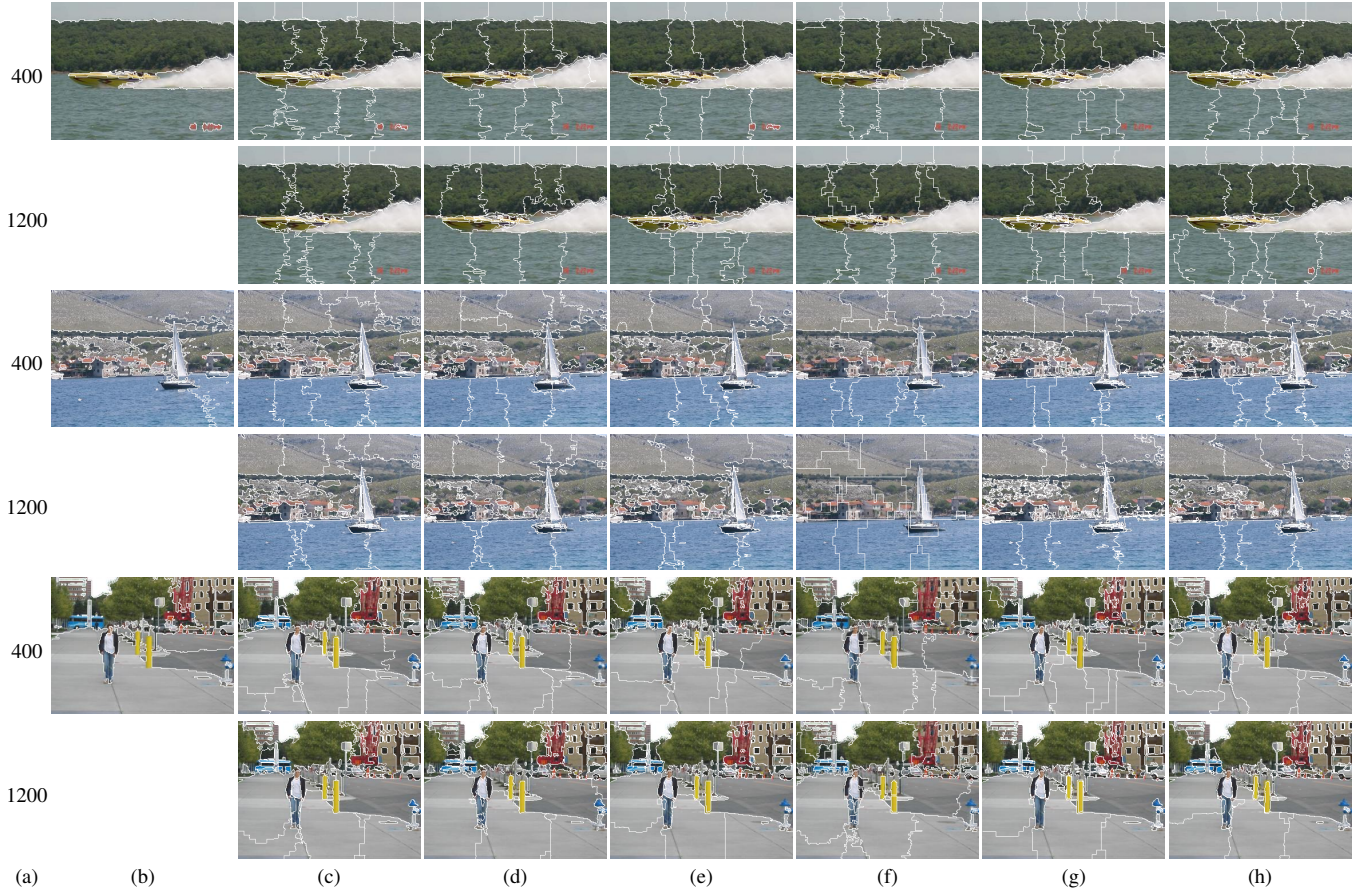
Fig. 16. (a) The number of superpixels generated before applying mean shift for image segmentation. (b) Segmentation results by applying the mean shift algorithm to image pixels directly. (c) ~ (h) Segmentation results by applying the mean shift algorithm to superpixels generated by (c) USEAQ, (d) USEQ, (e) SLIC, (f) SEEDS, (g) ETPS, and (h) LSC, respectively.
