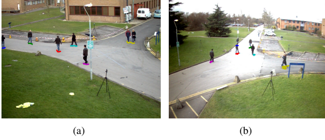
Fig. 4. Blob mapping on the ground plane: (a) the bottom boundaries of the blobs; (b) their mappings.
