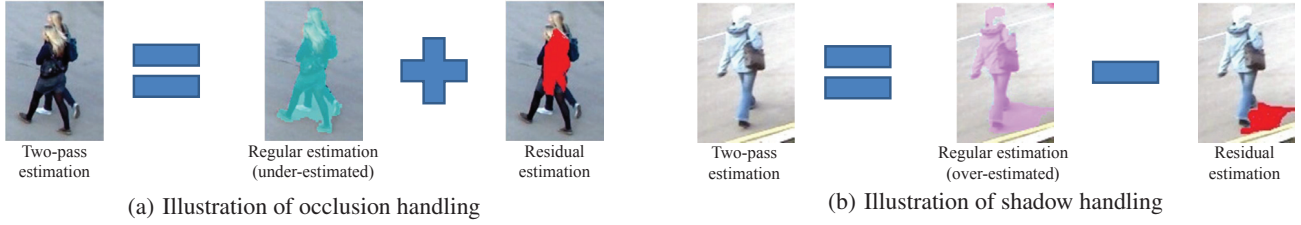
Figure 6: Our two-pass regression framework consists of a regular estimation and a residual estimation. While the former infers the number of people of a blob based using intra-camera low-level features, the later estimates the residual by exploiting inter-camera information. Fusing both together compensates for the difference between the ground truth and the estimated value, thus yielding higher accuracy than either.
