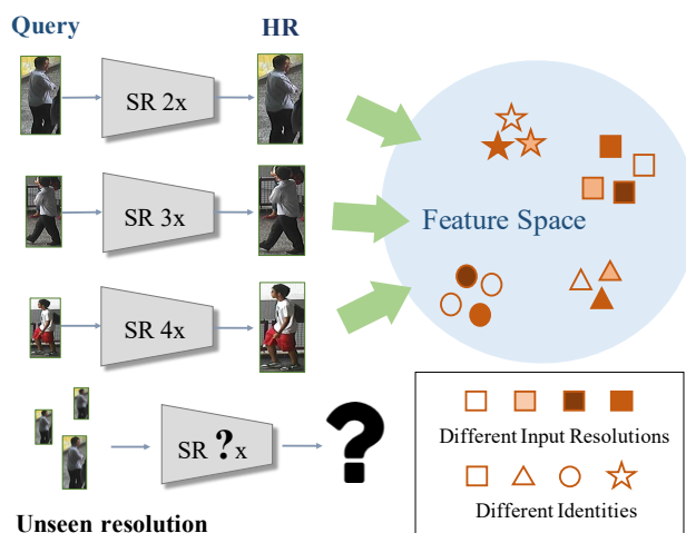
Figure 1: Illustration and challenges of cross-resolution person re-ID. Note that existing approaches typically leverage SR models with pre-selected resolutions followed by person re-ID modules. This cannot not be easily applied to query images with varying or unseen resolutions.
