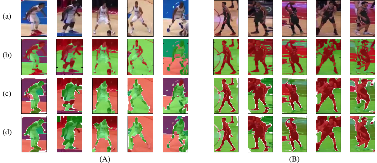
Fig. 3. (A) and (B) Two examples of the segmentation results. (a) The five bounding boxes of the players in a team. Segmentation results by (b) spectral clustering [20], (c) co-segmentation algorithm [16], and (d) our approach.
