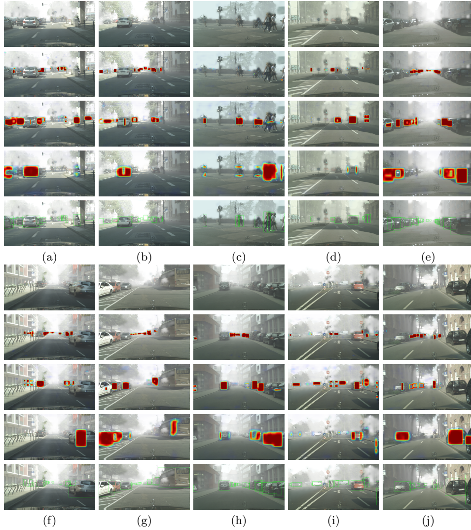
Fig. 2. (a) ~ (j) Ten examples of the response maps and detection results when adapting Cityscapes to Foggy Cityscapes. From top to bottom for each example, the input images, the corresponding response maps extracted from the feature layers F_3 \sim F_5 , and the corresponding detection results are shown, respectively.
