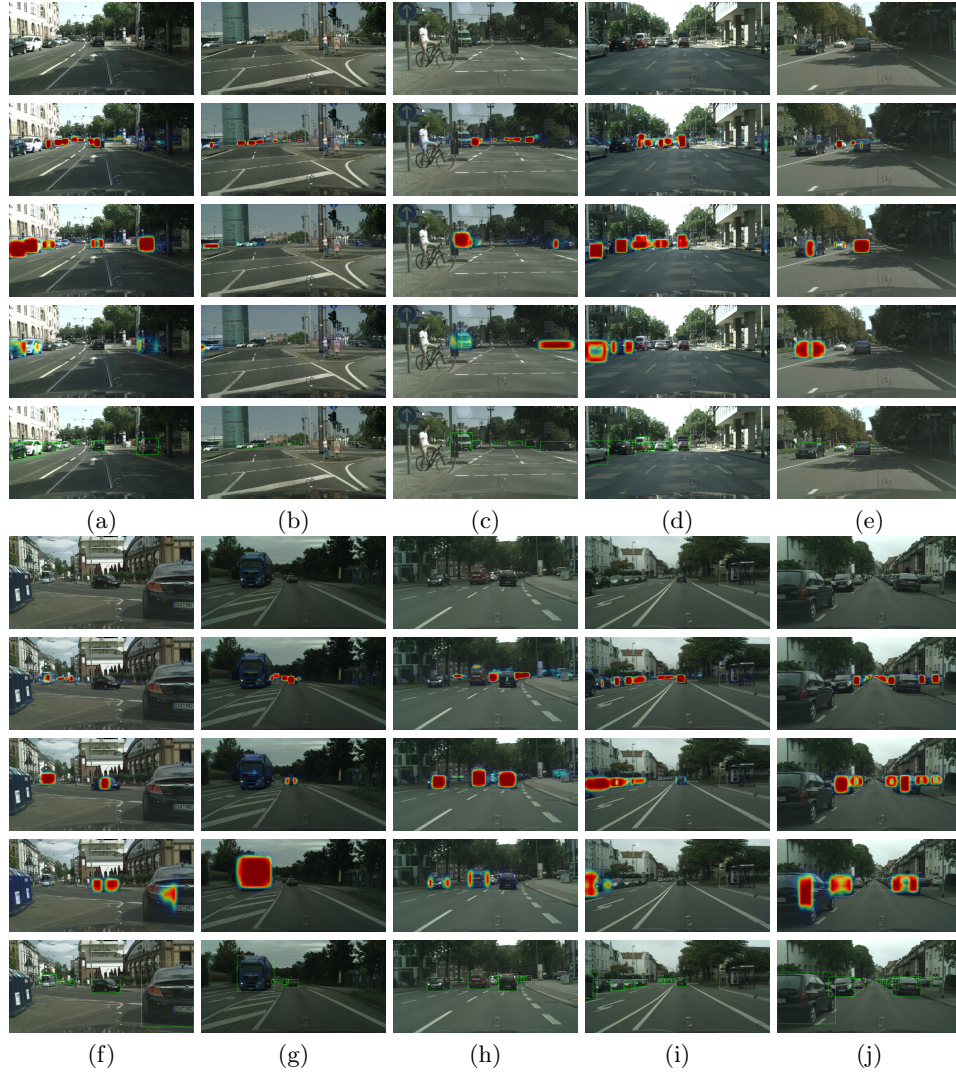
Fig. 3. (a) ~ (j) Ten examples of the response maps and detection results when adapting Sim10k to Cityscapes. From top to bottom for each example, the input images, the corresponding response maps extracted from the feature layers F_3 \sim F_5 , and the corresponding detection results are shown, respectively.
