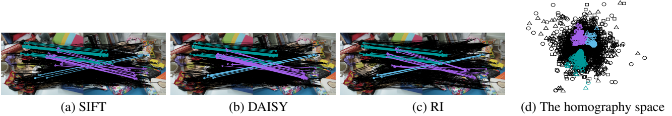
Figure 1. (a)-(c) are the matching results of SIFT, DAISY and RI, respectively. (d) gives the 2D visualization of correspondences in the homography space via classical multi-dimensional reduction [8]. Each correct matching is colored according to the common object it resides in, and wrong matchings are in black.
