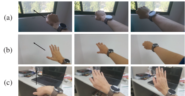
Figure 1: Gestures of categories (a) fist , (b) fetch , and (c) palm-up . Visual modalities are effective to separate gestures of category fist from the rest owing to their distinctive hand shapes. In contrast, motion-based modalities are discriminative for gestures of category palm-up due to the consistent moving trajectories. Meanwhile, gestures of class fetch are better predicted by using both types of modalities jointly.
