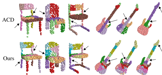
Fig. 10. Decomposed point clouds obtained via ACD [81] (top) and our method (bottom) that are utilized to perform semi-supervised part segmentation reported in Table VII. The arrows indicate major differences between the two methods.
