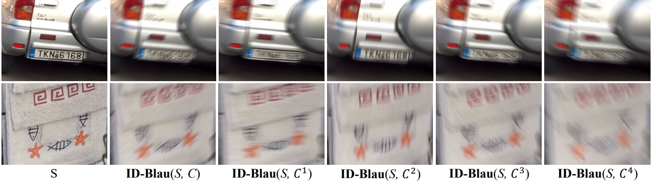
Figure 4. Illustration of reblurred images with ID-Blau. It takes a sharp image S and a blur condition map C = [x; y; z] as inputs to generate the corresponding blurred image. We show several generated blurred images by altering C , such as unit horizontal or vertical blur orientations, C^1 = [1; 0; z] and C^2 = [0; 1; z] , horizontally inverse C as C^3 = [-x; y; z] , and C^4 = [-x; y; 2z] with twice the magnitude for C^3 .
